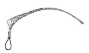
Double Weave, Long Length, Closed Mesh, Offset eye. Cable Diameter - 2.000-2.490-inch, Cable Diameter - 27-inch, Break Strength- 11,000 lbs.
