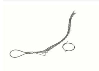
Double Weave, Long Length, Split Lace, Offset Eye. ◆ Cable Diameter - 1.000-1.240\'\', Mesh Length - 21\'\', Break Strength - 4,100 lbs.
