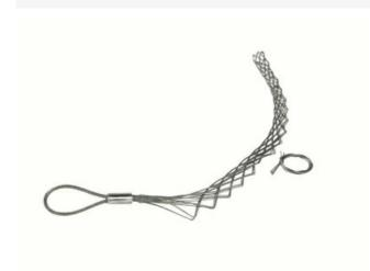
Double Weave, Standard Length, Split Lace, Offset Eye. ◆ Cable Diameter - 1.500-1.740\'\', Mesh Length - 18\'\', Break Strength - 5,500 lbs.
