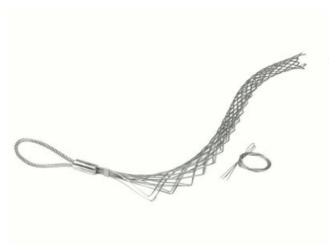
Double Weave, Standard Length, Split Lace, Offset Eye. ◆ Cable Diameter - 1.750-1.990\'\', Mesh Length - 19\'\', Break Strength - 7,300 lbs.
