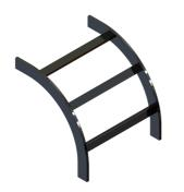
Radius curved runway permits smooth vertical to horizontal transitions. Stringers are 1-.5 in x .375 in steel tubes; cross slats are 1 in x .5 in x .125 in steel tubes. UL listed.
