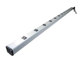
Twelve outlets, rugged gray aluminum housing, 15A, lighted switch, 6' [1.8m] 14/3 SJT black cord with NEMA5-15 plug. Length 72'' [1.8m]. Receptacle center-to-center 5 1/4'' [133mm]. Snap-on, slide-off mounting.
