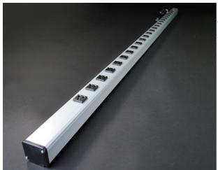
Twenty-four outlets, rugged gray aluminum housing, 15A, lighted switch, 6' (1.8m) 14/3 SJT black cord with NEMA5-15 plug. Length 72'' (1.8m). Receptacle center-to-center 2 1/2'' (64mm). Snap-on, slide-off mounting.
