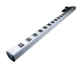
Sixteen outlets, lighted switch, rugged gray aluminum housing, 15A, 6' [1.8m] 14/3 SJT black cord with NEMA5-15 plug. Length 48" [1.2m]. Receptacle center-to-center 2 1/2" [64mm]. Snap-on, slide-off mounting.
