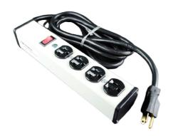
Four 20A, 120V, 60Hz, 2500 watt outlets, lighted switch, putty white aluminum housing, 15' (4.6m) 12/3 SJT black cord with NEMA5-20 plug. Length 10 3/4" (273mm). Receptacle center-to-center 1 1/2" (38mm). Snap-on slide-off mounting.
