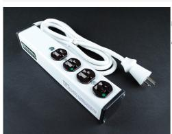
Four outlets. Rugged white aluminum housing. 15' (4.6m) 14/3 SJT white cord with NEMA5-15 plug. Length 10 3/4" (237mm). Receptacle center-to-center 1 1/2" (38mm). Snap-on, slide-off mounting. Not for use in critical care enviornments. NOTE: Not for use where Article 517 of NEC requires Hospital Grade Outlets.
