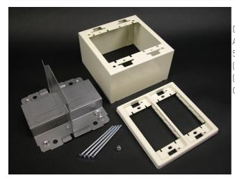
Divided, two-gang, labor saving, over-the-raceway device box. Allows both power and low voltage at a single point-of-use. Accepts 5507 Series Faceplates, Ortronics TracJack and Series II Modules (requires S2-EPL Plate), Pass and Seymour Activate Series Inserts (requires CM-EPLA Plate), and Wiremold Open System Communication Modules (requires CM-EPLA Plate).
