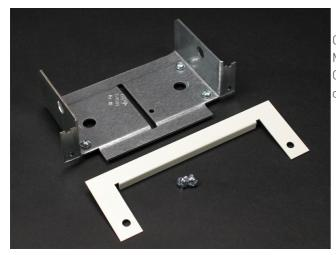
Connects 4000 Series Raceway to surface type panel boxes. Maintains maximum wire capacity of 4000 Series Raceway. Separate C-shaped flange fits around raceway, to hide irregularities made during cutting into box.
