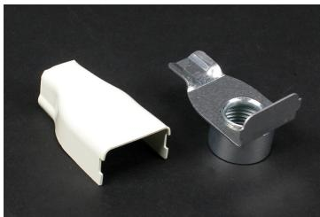
Connects raceway at right angles to 1/2" trade size conduit or armored cable connectors. When used with 700 Series Raceway, break out crescent twistout in cover.
