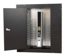
The EN-RPA18R120-347V is an addressable lighting control panel that allows each relay to be individually controlled and configured to best meet the needs of the facility. Energy management strategies such as smart time scheduling, occupancy control, and daylight harvesting can be deployed through the use of the Relay Panel. Each relay can be addressed as an individual zone or as part of a larger zone and is controlled through Polaris software.
