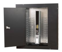
The EN-RPA0R120-347V is an addressable lighting control panel that allows each relay to be individually controlled and configured to best meet the needs of the facility. Energy management strategies such as smart time scheduling, occupancy control, and daylight harvesting can be deployed through the use of the Relay Panel. Each relay can be addressed as an individual zone or as part of a larger zone and is controlled through Polaris software.
