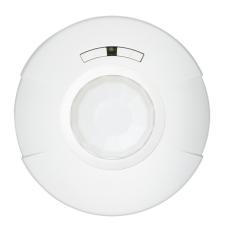
The EN-SCPPH-0450-GB2 is a ceiling/surface mount sensor that combines both Passive Infrared (PIR) and Photocell sensing into a single device. With a range of 450 sq. ft., the GreenBus sensor connects to the Wattstopper PLUS system through a GreenBus cable with a standard 2-pin connector.
