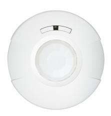
The EN-SCPPH-1500-GB2 is a ceiling/surface mount sensor that combines both Passive Infrared (PIR) and Photocell sensing into a single device. With a range of 1500 sq. ft., the GreenBus sensor connects to the Wattstopper PLUS system through a GreenBus cable with a standard 2-pin connector.
