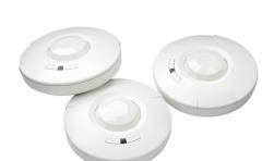
The EN-SCPPH-1500-ZB is a ceiling/surface mount sensor that combines both Passive Infrared (PIR) and Photocell sensing into a single device. With a range of 1500 sq. ft., the Wireless Sensor connects to the Wattstopper PLUS system via Zigbee
