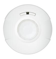
The EN-SCPPH-HB-GB2 is a ceiling/surface mount sensor that combines both Passive Infrared (PIR) and Photocell sensing into a single device. With a variable coverage range from approximately 1,100 sq. ft. to 2,800 sq. ft. (depending on mounting height), the GreenBus sensor connects to the Wattstopper PLUS system through a GreenBus cable with a standard 2-pin connector.
