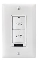
Legrand's series wall switches are low voltage device for manual control of shades in one or more locations. This device has 1 or more buttons and can control any shade motors connected to DLM shade controllers. The switches connect using standard DLM IRB RJ45 cables and have a counter balanced design that allows shades to be pulled into position from the hembar.
