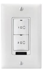
Legrand's series wall switches are low voltage device for manual control of shades in one or more locations. This device has 1 or more buttons and can control any shade motors connected to DLM shade controllers. The switches connect using standard DLM IRB RJ45 cables and have a counter balanced design that allows shades to be pulled into position from the hembar.
