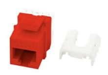
Easily terminate all four pairs using Legrand Punchdown tool (Part Number AC3400) RJ45 Inserts can be terminated with any 110 punchdown tool Exceeds EIA/TIA 568A/B Cat5e Performance Specifications Available in Black, Brown, White, Light Almond, Grey, Blue, Orange, Ivory and Red Contractor packs available in quantities of 50. To order, use part number WP3475-LA-50
