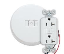
Wireless Receptacle Controls facilitate occupancy-based AutoOn/Auto-Off control of plug loads without the need to wire receptacles to room controllers. A WRC transmitter works with WRC RF-enabled relay-controlled receptacles.
