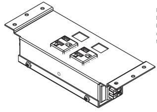
Kit contains two 4 wire, 2 circuit connectorized cables each 27" in length (one M/F and one F/F) with black cable covers and 4 cable clamps for mounting, one black work surface portal with 2 power and 2 keystone openings for communications. Portal is wired for circuit 1. For circuit 2 wired portals, order the "-2" suffixed part number.
