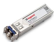
Alcatel SFP-GIG-BX-D-80 Compatible 1000Base-BX SFP Transceiver (SMF, Tx: 1550nm Rx: 1490nm, 80km, LC Duplex, DDM, I-Temp)
